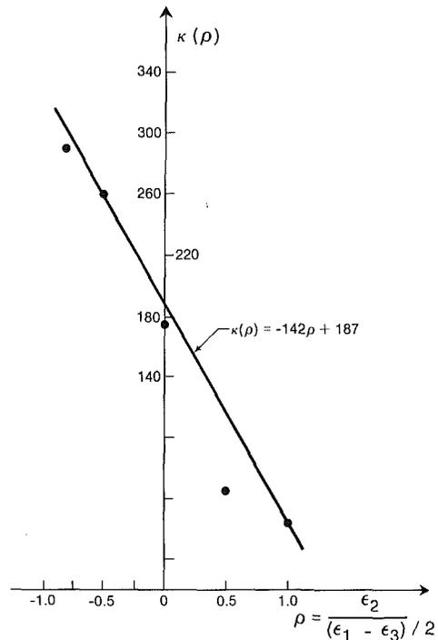
Fig. 4 Strain ratio function  $\kappa(\rho)$  versus strain ratio for biaxial tests
