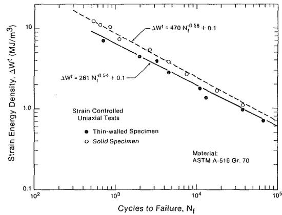
Fig. 3 The total strain energy density versus number of cycles to failure of thin-walled [8, 27] and solid round specimens [14] for uniaxial loading
