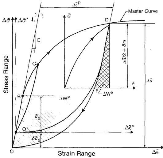
Fig. 2 The coordinate system for the master curve
