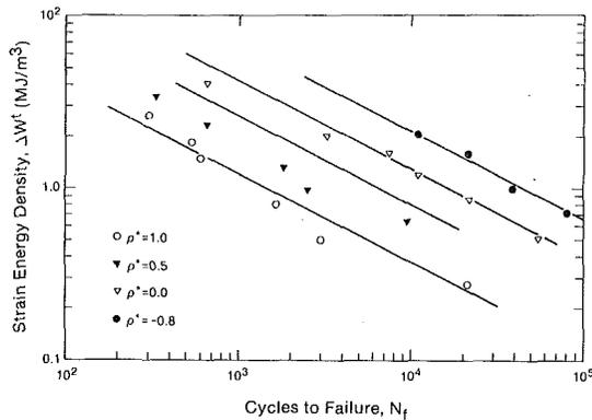
Fig. 5 The predicted strain energy density  $\Delta W^t$  versus the number of cycles to failure,  $N_f$ , for various strain ratios, and the experimental data from reference [27]
