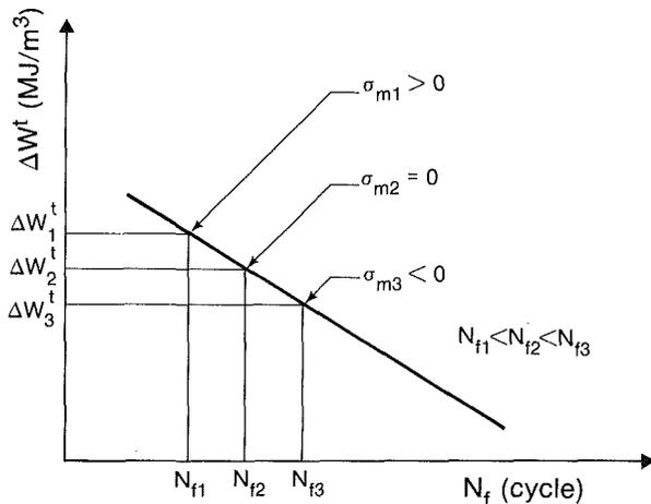
Fig. 6 The effect of mean-stress as predicted by the present theory
