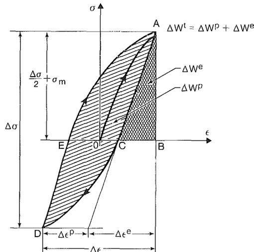
Fig. 1 Elastic and plastic strain energy densities for a uniaxial cyclic loading case
