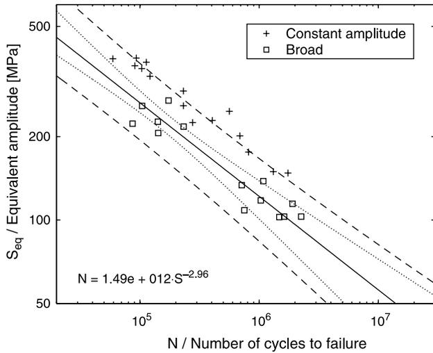
Fig. 4. *SN*-curve estimated from Broad spectrum tests, with prediction and confidence bands for constant amplitude.
