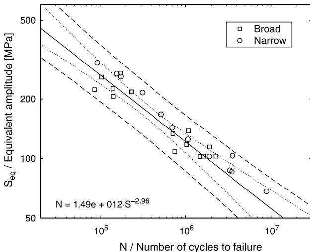
Fig. 5. *SN*-curve estimated from Broad spectrum tests, with prediction and confidence bands for Narrow spectrum.
