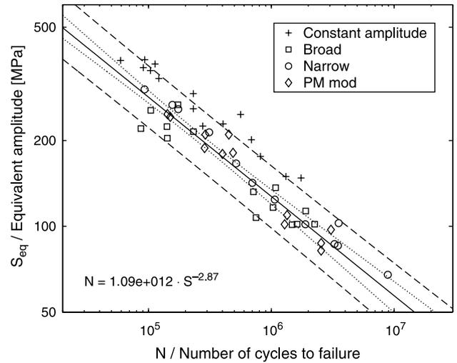
Fig. 6. *SN*-curve estimated from all variable amplitude tests, with prediction and confidence bands for constant amplitude.
