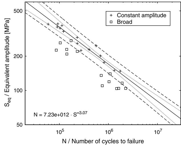
Fig. 3. *SN*-curve estimated from constant amplitude tests, with prediction and confidence bands for Broad spectrum.
