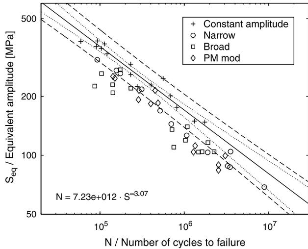
Fig. 2. *SN*-curve estimated from constant amplitude tests, with prediction and confidence bands for constant amplitude loads. The lives for the Broad, Narrow, and PM mod spectra tests are plotted versus the equivalent loads calculated using the estimated  $\beta$ .
