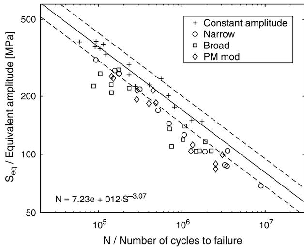
Fig. 1. SN-curve estimated from constant amplitude tests, with scatter bands of two standard deviations. The lives for the Broad, Narrow, and PM mod spectra tests are plotted versus the equivalent loads that are calculated using the estimated  $\beta$ .
