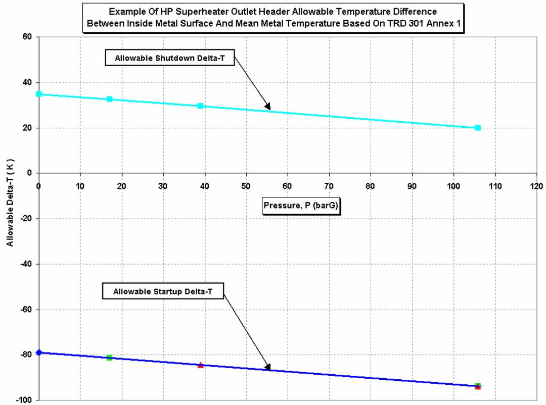
**Figure 5: Example Allowable Delta-T Curves For Startup And Shutdown Of A HP Superheater Outlet Header.**
