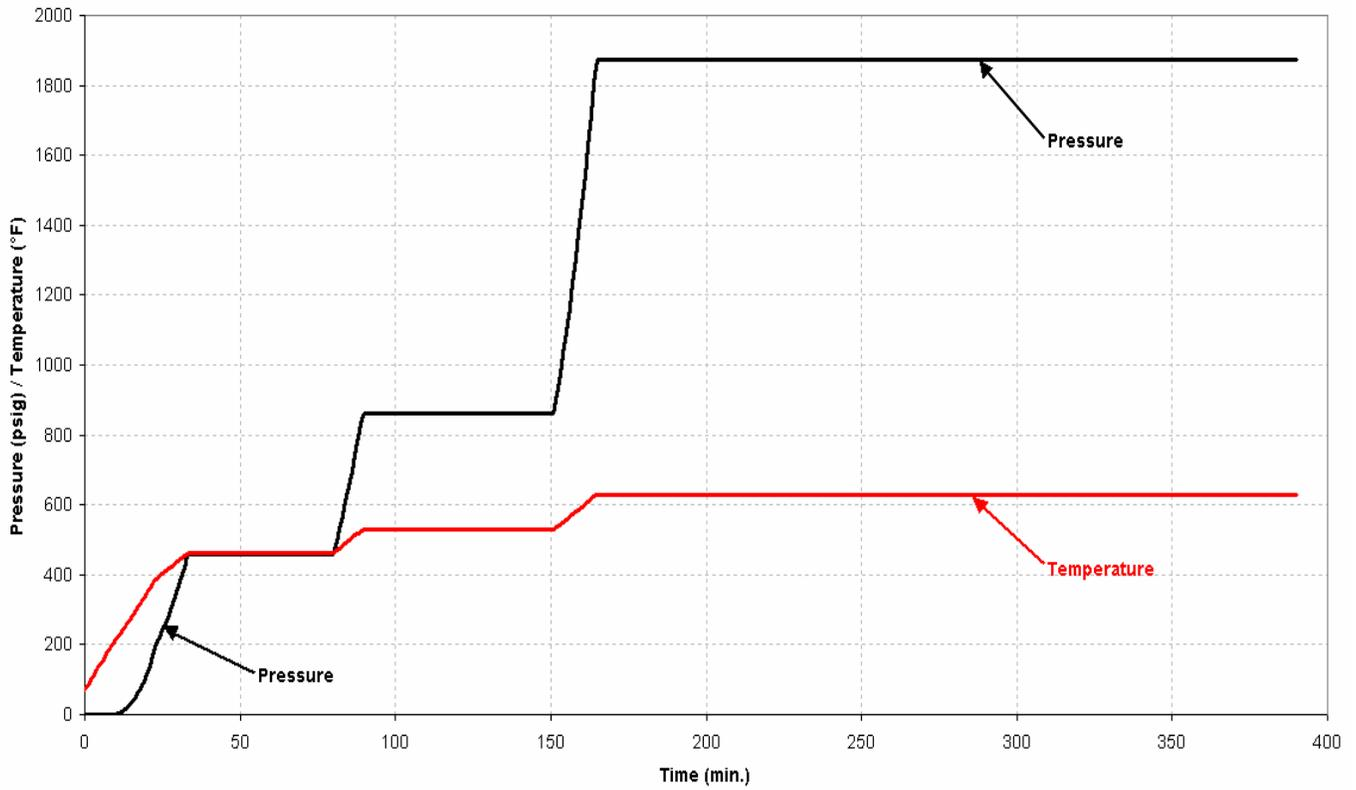
Figure 1: Typical Cold Startup Curve For HP Steam Drum Downcomer Nozzle
