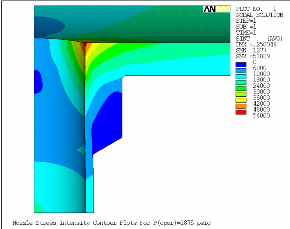
**Figure 3: Example Of Stress Intensities From Finite Element Analysis Of Downcomer Nozzle In HP Drum Due To Operating Pressure**
