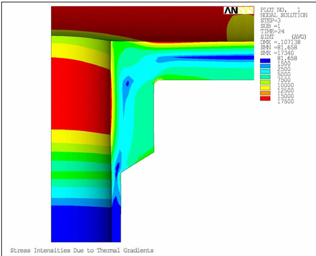
**Figure 4: Example Of Stress Intensities From Finite Element Analysis Of Downcomer Nozzle In HP Drum Due To Thermal Gradients At Cold Startup**
