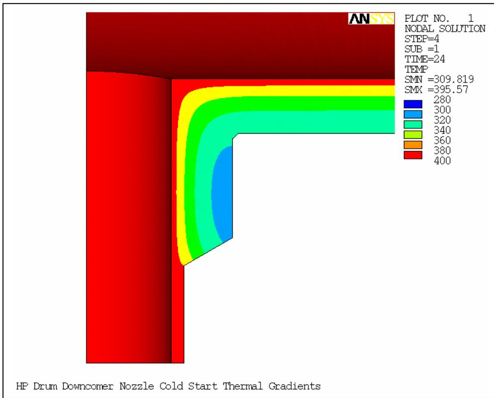
Figure 2: Example Of Thermal Gradients From Finite Element Analysis Of A Downcomer Nozzle In A HP Drum During Cold Startup
